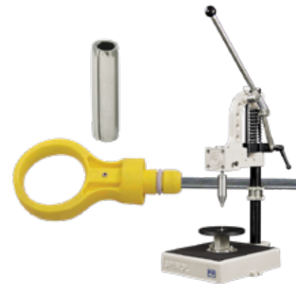
A Light Duty Coiled Pin retains the plastic ring to the metal rod of an automotive dip stick. These pins can be easily installed with SPIROL's Model PM Manual Pin Inserter.
